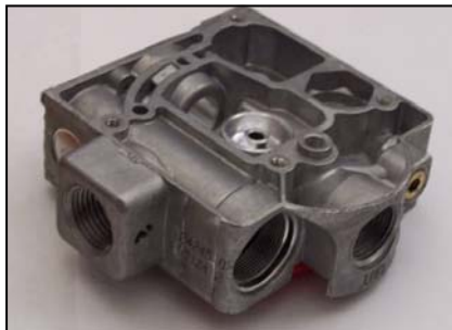
Aluminium casting awaiting thread check
